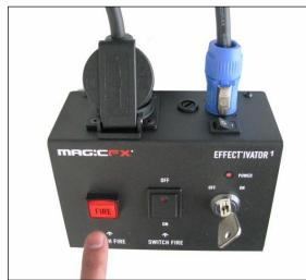
To operate the CO2 Power Jet you press the switch on and off. As soon as you press the switch the magnetic valve will immediately open and a white smoke plume will exit from the CO2 Power Jet. When you press the switch again to the off position the valve will immediately close.
