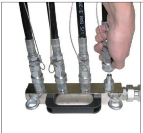
Connect the other ends of the CO2 high pressure hoses to the distribution block and check that these are properly connected.
