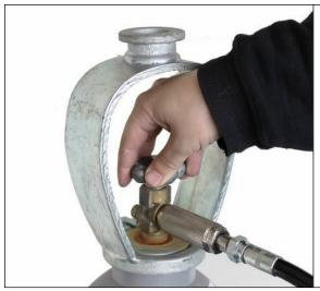
When the system is properly connected you can open the valve of the CO2 bottle. Check for leaks.
